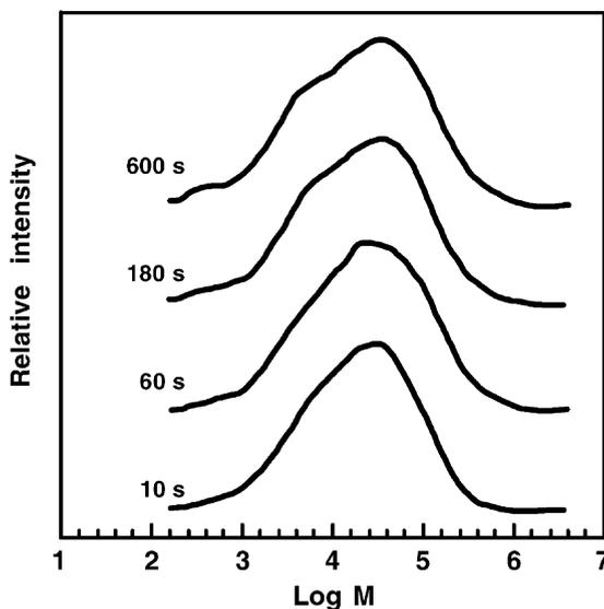
Fig. 2. Dependence of GPC curves on catalyst pretreatment time for polypropenes obtained in stopped-flow polymerization with the TEA-pretreated  $\text{TiCl}_4/\text{DBP}/\text{Mg}(\text{OEt})_2$  catalysts. TEA pretreatment time: 10, 60, 180 and 600 s.
