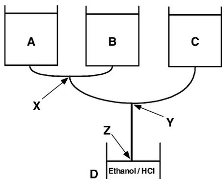
Fig. 1. Schematic illustration of the modified stopped-flow apparatus for TEA pretreatment and propene polymerization of the  $\text{TiCl}_4/\text{DBP}/\text{Mg}(\text{OEt})_2$  Ziegler–Natta catalyst (A–C: vessels with water jacket; D: ethanol with HCl as a quenching agent; X and Y: three-way Teflon taps).
