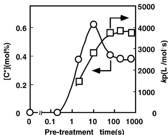
Fig. 3. Dependence of active sites concentration  $[C^*]$  (○) and chain propagation rate constant  $k_p$  (□) on catalyst pretreatment time in stopped-flow propene polymerization with the TEA-pretreated  $TiCl_4/DBP/Mg(OEt)_2$  catalysts.
