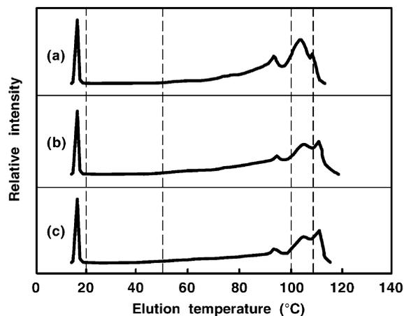
Fig. 4. Dependence of TREF profiles on catalyst pretreatment time for polypropenes obtained in stopped-flow polymerization with the TEA-pretreated  $TiCl_4/DBP/Mg(OEt)_2$  catalysts. TEA pretreatment time: (a) 10 s; (b) 60 s; (c) 600 s.
